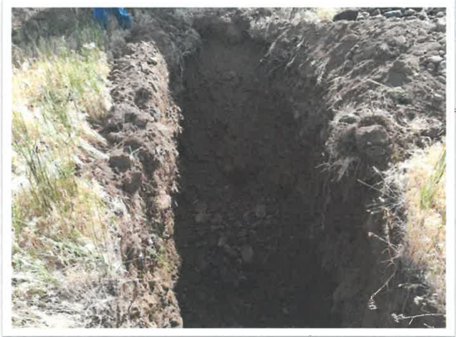
Photo 2 – Test Pit showing soil profile
